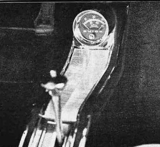
GS 400 optional console holds shifter and extra-cost, out-of-easy-sight, tachometer
