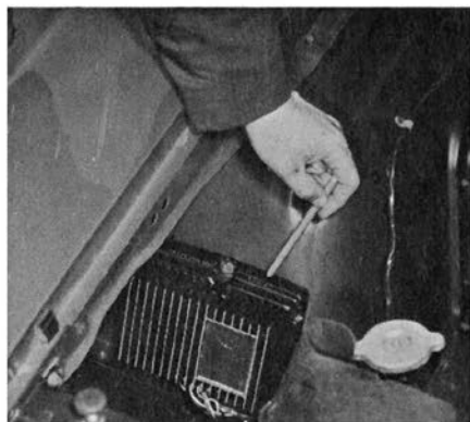
New UHV capacitive discharge ignition works with a pointless distributor.
