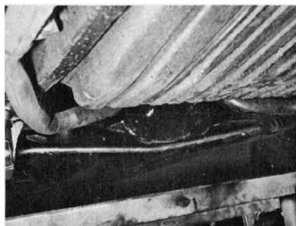
Rear sway bar is 4-4-2 exclusive, key to car's precise handling qualities.
