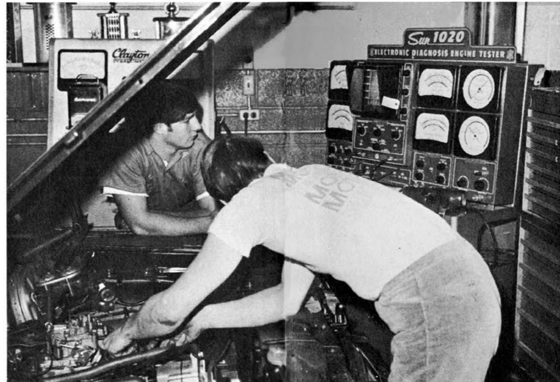
Test car was set up on a Clayton dyno using the latest Sun 1020 scope.
