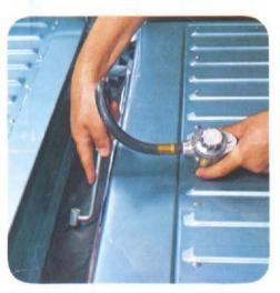
AIR-BOOSTER SHOCK ABSORBERS at the rear are standard. Air pressure can be adjusted for road and load conditions.
