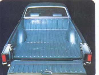
CARGO BOX is strong and spacious with room for objects more than six feet long. Reinforced steel floor and double sidewalls take the knocks on the inside without marring exterior beauty.
