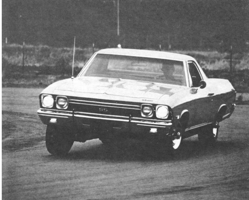
CORNERING power is high, even with the big engine. El Camino understeers at steady cornering speeds, but the car can be balanced with more power.
