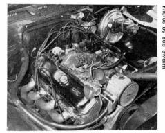
Meet the L-34 version of Chevrolet's 396 cubic inch "Rat Motor." About all we did to our 350-horse powerplant was install a set of Cyclone's fine exhaust headers.
