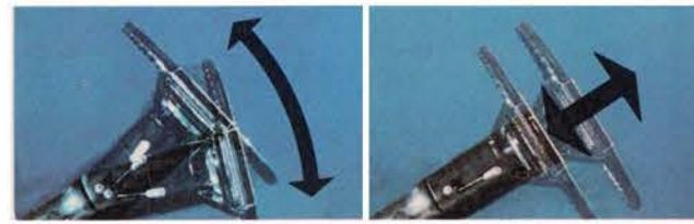
Like things just so? Tilt-and-Telescope Steering Wheel adjusts to driver's size with 3-inch in-out adjustment, 7 up-down positions. Makes for easier entry and exit, too!
