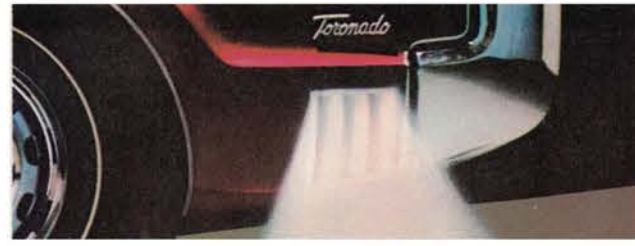
Take a corner with confidence! Cornering lights operate automatically when you use directional signals with lights on—assure more convenient turning at night.
