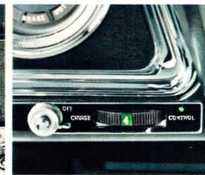
Cruise-Control —Set your speed and Cruise-Control maintains it, while reducing fatigue. Has built-in resistance when set speed is reached, acts as warning device. Extra cost option on all models.
