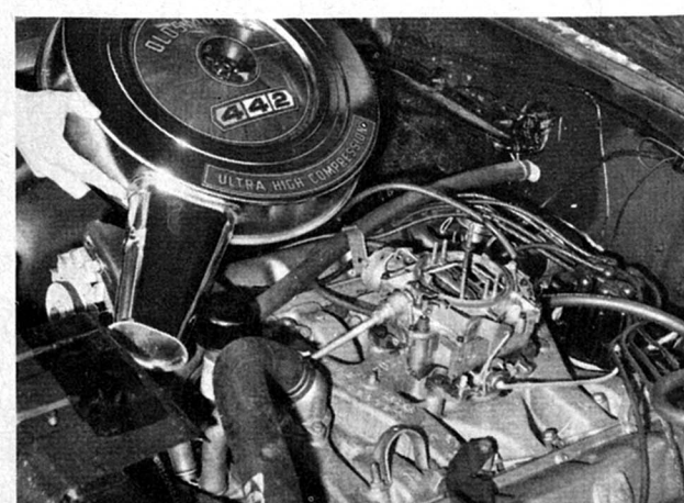
Beefy 400 cube mill sports a large four-barrel and a top notch porting layout. It should be a strong contender in Stock competition. Wire wheel disc and performance tires hide the oversize 9½-inch finned drum brakes from view.
