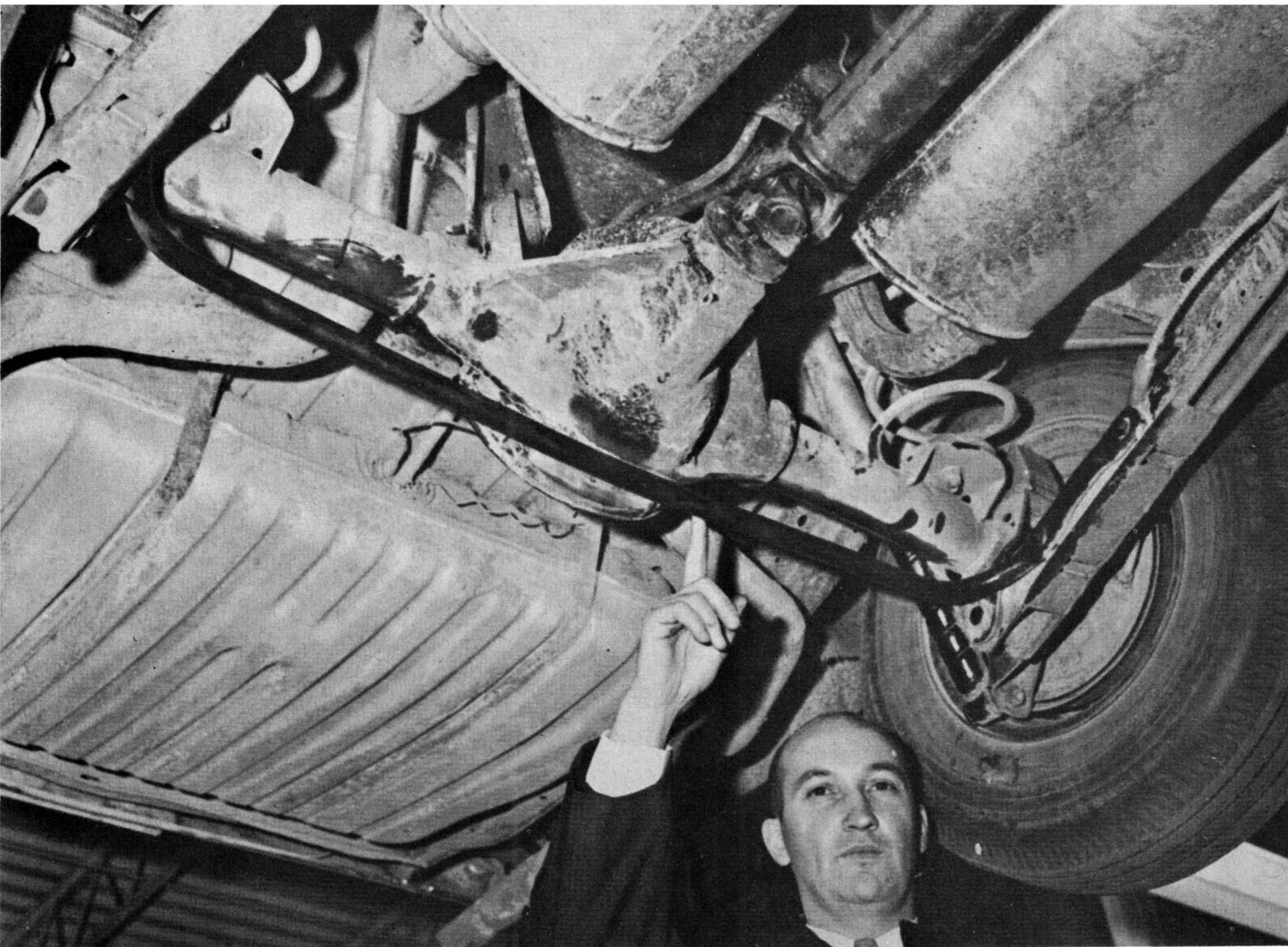
Rear stabilizer bar is bolted directly to the lower control arms. Limited slip rear houses 3.55 to 1 gears.
