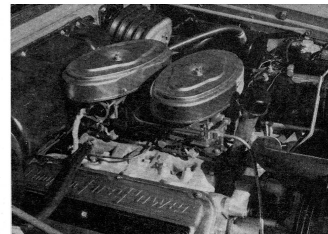
TINY AIR FILTERS on the 300-D dual Carters are designed to produce throaty power throb at full throttle.
