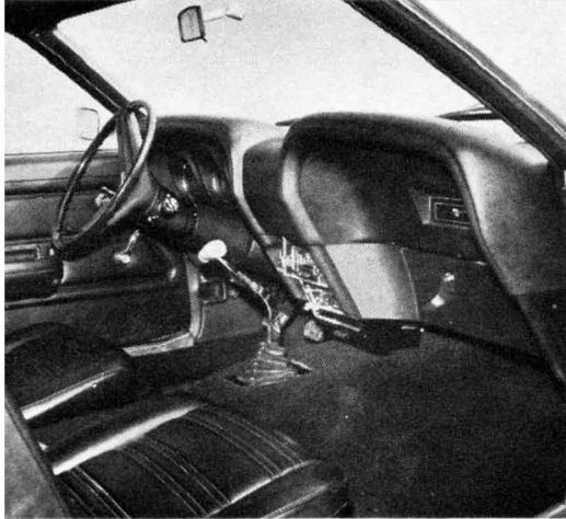
Hurst T-handled shifter comes with stock 4-speed. Interior is spartan but not uncomfortable. More gauges are needed.
