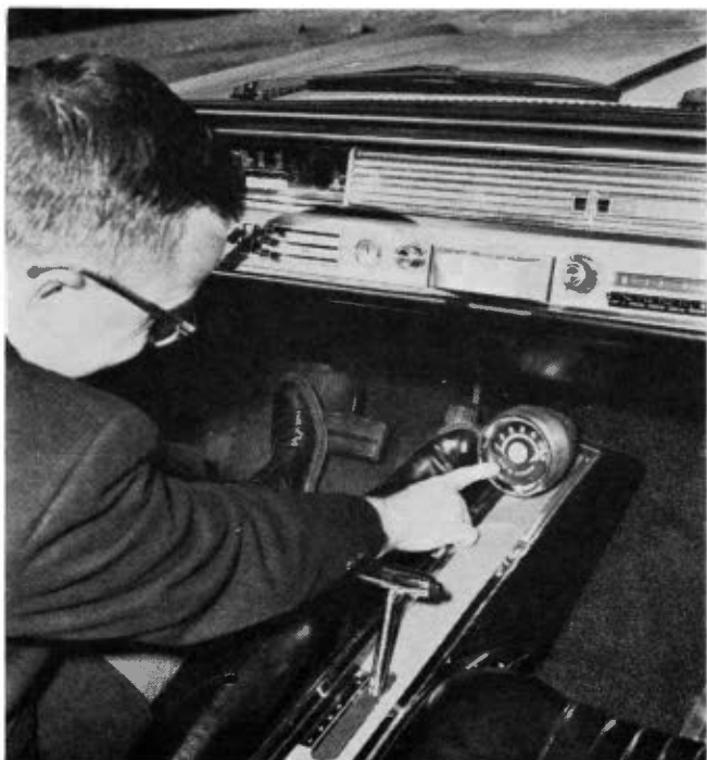
Tach remains only a handsome ornament, since its location made it almost impossible to see. T-bar shift and console are options.
