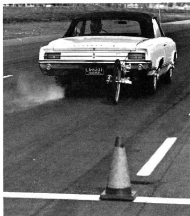
Panic stops caused left rear wheel to lock up first, but under normal conditions, it took lots of abuse to bring out brake fade.
