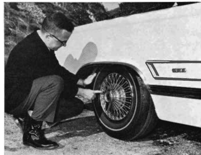
Optional wire wheel covers may look sharp, but they add weight and when fitted make it impossible to check tires or add air.
