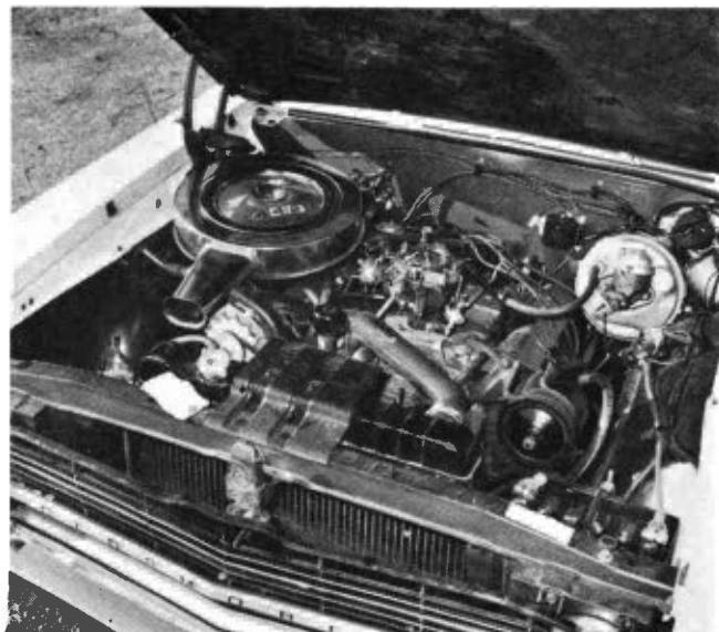
Husky 345-hp powerhouse gets extra cooling from heavy-duty radiator. V-8 purrs on two throats — really charges on four.
