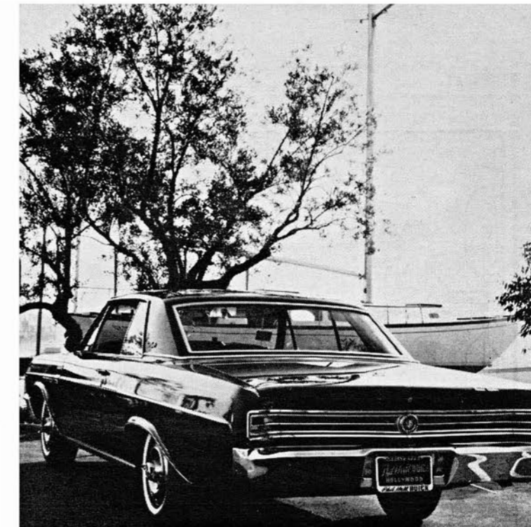
WALL-TO-WALL taillights are distinctive feature of Skylark styling, but turned out to be completely invisible from the sides.
