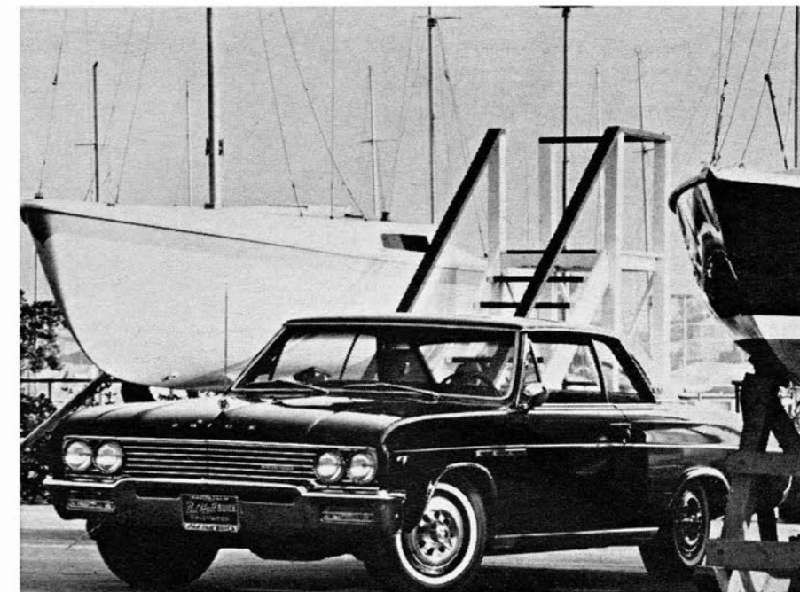
BRIGHT METAL trim is cleaned off the sides for the Gran Sport package. Simulated "ventiport" plate replaces fore-to-aft sweep spear.
