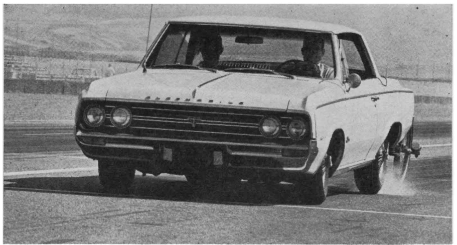
Cutlass' left rear wheel always locked up first and was tough to unlock, yet stopping power was consistently strong and swerve-free, giving us a number of stops before fading.
