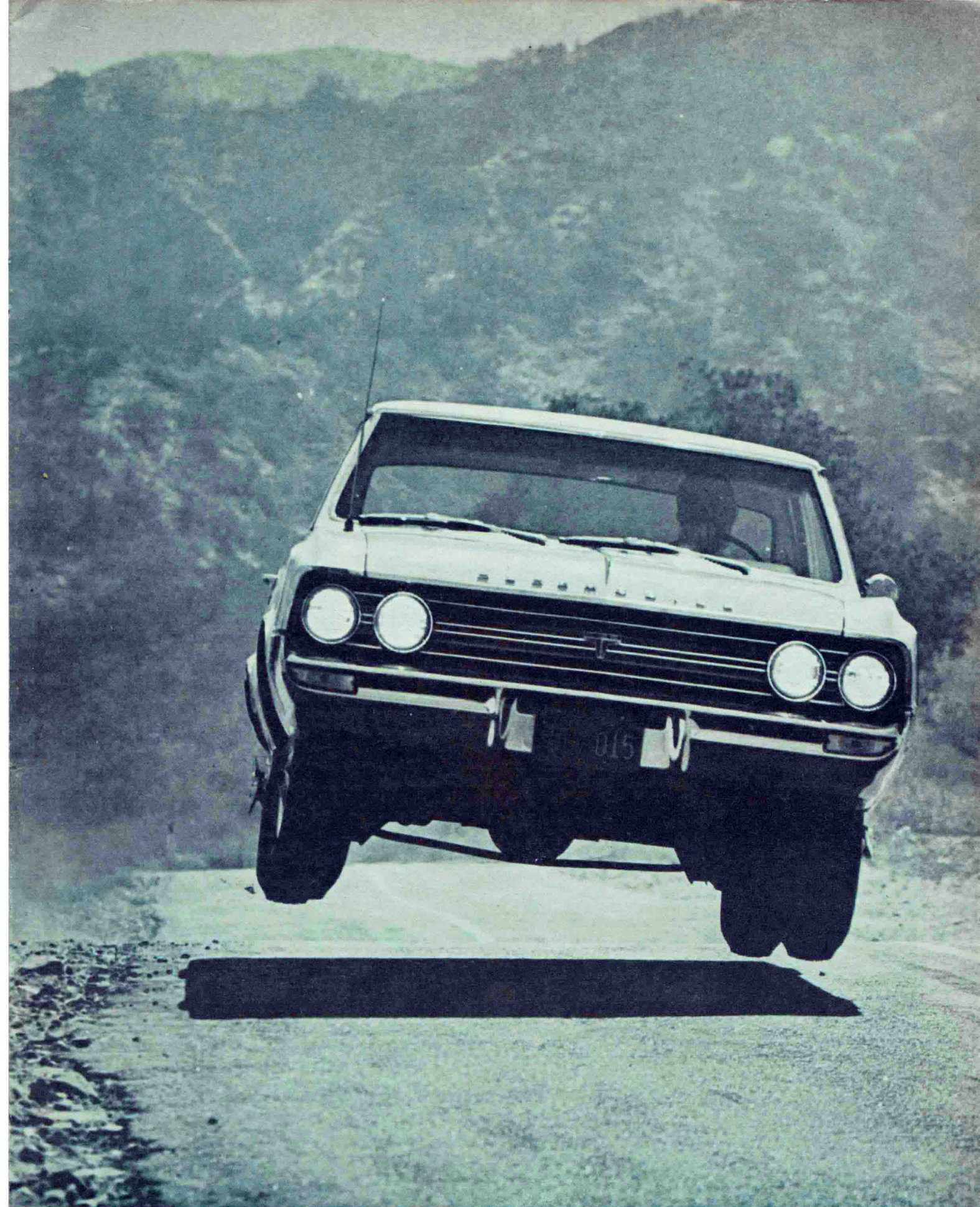
F-85's heavy-duty suspension would bottom, but only when thrown through high-speed dips like this at 65+ mph. Special rear anti-
