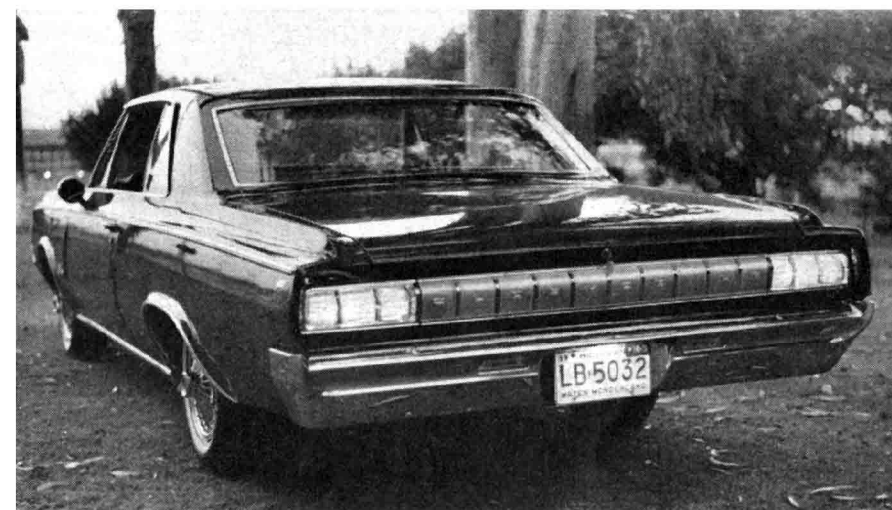
TWO-DOOR hardtop has normal rear window although 4-door sedan is fitted with stylish concave glass à la Starfire.
