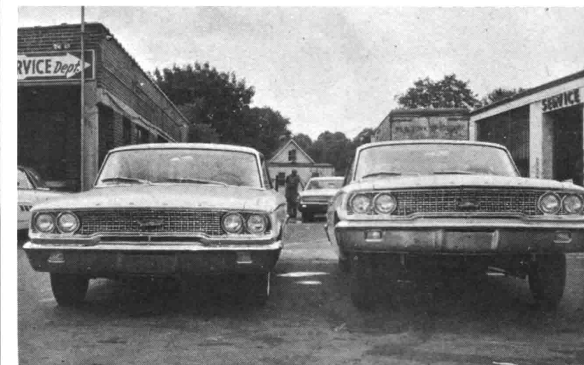
A comparison of the stock Galaxie and dragging version indicates the modifications that were made to the 'glasser's shocks, springs, stabilizer bar.
