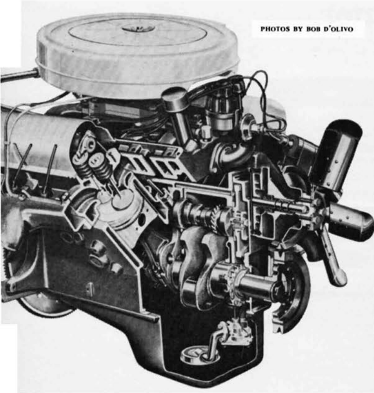
Well proven 390-cubic-inch engine, borrowed from the Thunderbird, is rated at 300 horsepower. Another variation of this engine (Police Performance) uses different camshaft to produce 330 hp.
