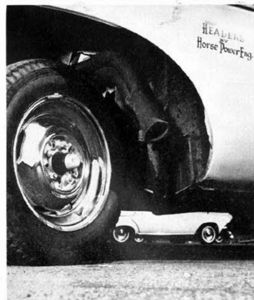
MODIFIED HEADERS vs. factory system: modified (left, below) dump out behind front wheel, factory type extend back under car.
