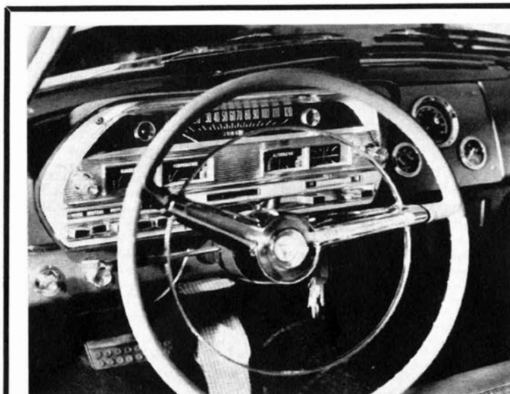
EXTRA INSTRUMENTS and foot-fitting throttle pedal were added to Golden's car. Instruments are tachometer, oil pressure and water temperature.
