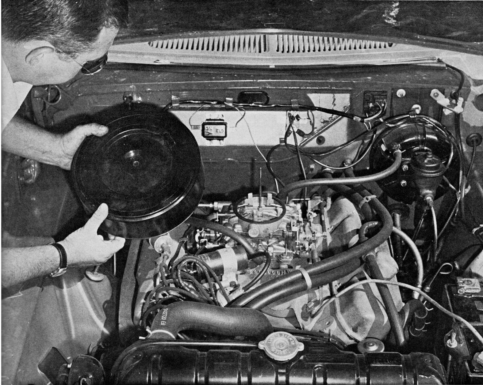
BIG 383-INCH GOLDEN COMMANDO V-8 USES SAME BLOCK AS "426" S/S. SMALL AIR CLEANER HAS PAPER ELEMENT, DOESN'T SILENCE.
