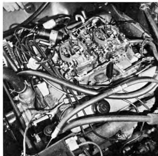
Progressive mechanical linkage is fitted and rear carb, which opens first, has automatic choke. Manual choke kit is available. Manifold (below) is of log type with four barrels of one side feeding left bank and four barrels of other side feeding the right bank.
