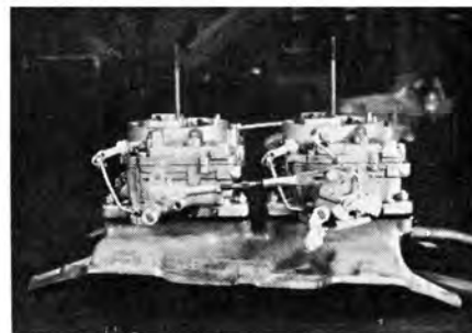
Progressive mechanical linkage is fitted and rear carb, which opens first, has automatic choke. Manual choke kit is available. Manifold (below) is of log type with four barrels of one side feeding left bank and four barrels of other side feeding the right bank.
