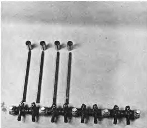
Beefy pushrods and adjustable cast rocker arms (above) are used with mechanical lifters. Shown at left, these parts were available through Chrysler Marine, but are now available from Chrysler car dealers as options.
