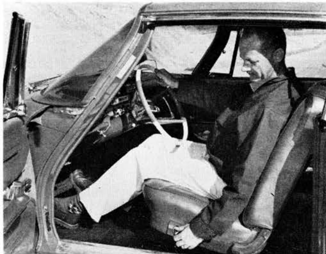
With a flick of a switch, the electrically powered seat tilts itself backward or forward, up or down, and adjusts for rake.
