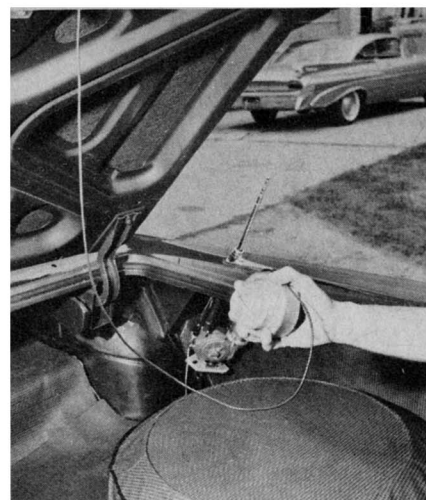
A neat option is the trunk compartment light with emergency extension cord.
