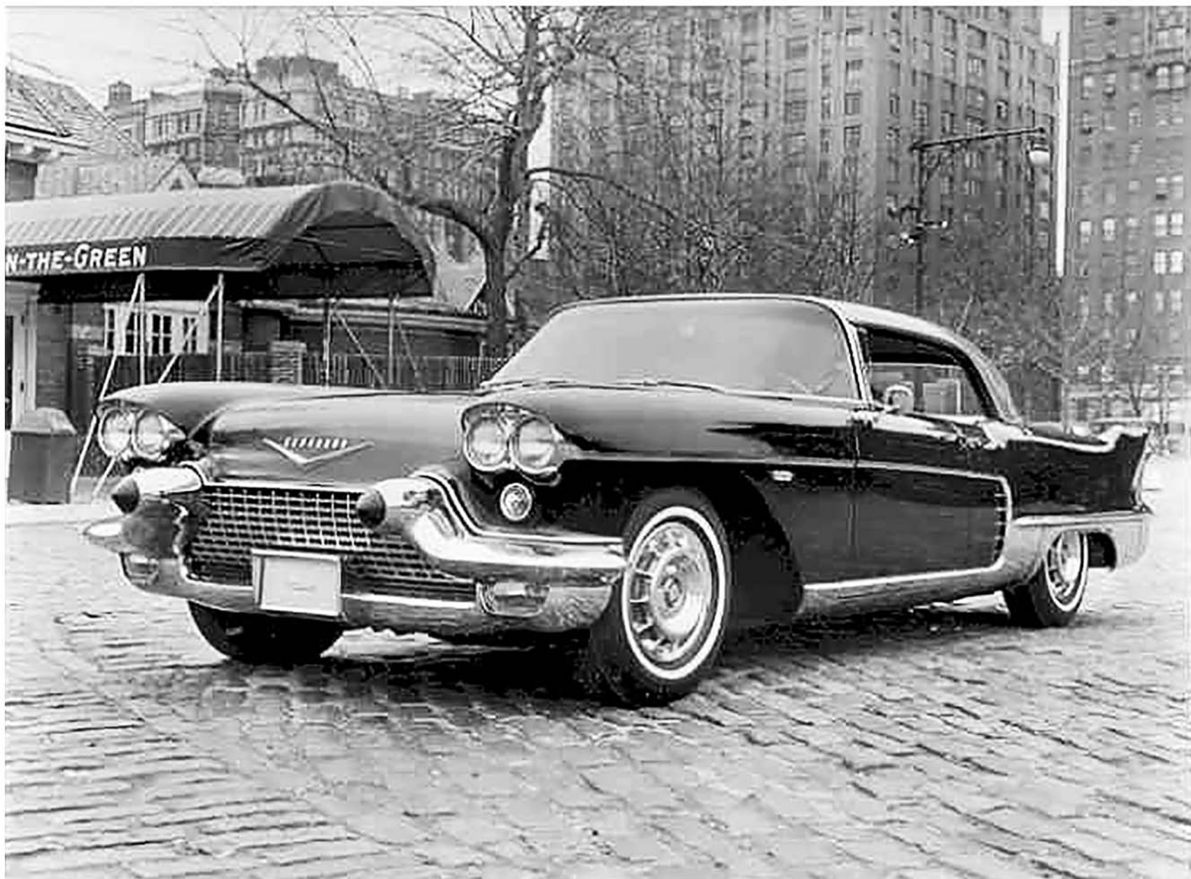
THE CADILLAC ELDORADO BROUGHAM -- This ultra luxury automobile features a true four headlamp system, which was pioneered by Cadillac. The Brougham is 55 1/2 inches high and has a length of 216 inches.
