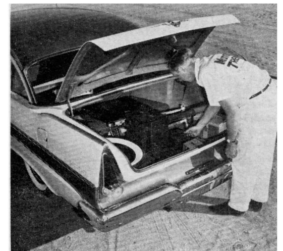
TORSION-BAR HINGE reduces interference with luggage to a maximum. Trunk is very deep, but not high, so spare is mounted flat. There is no water drain.
