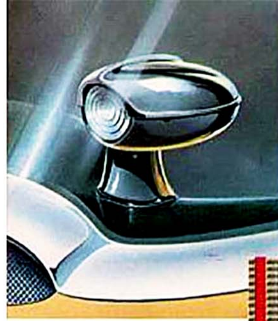
CADILLAC AUTRONIC-EYE* automatically dims the Cadillac's lights when a car is approaching, raises them after it has passed. An unusually popular feature, the Autronic-Eye takes much of the guesswork out of night driving.
