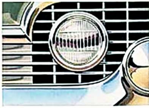
FOG LAMPS* for 1954 are an integral part of the grille assembly. When fog lamps are selected, the parking and turn-signal lights are incorporated in the unit.
