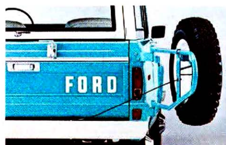
Swing-Away Spare Tire Carrier puts the spare tire out of the way for more cargo area, easier access.
