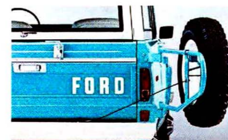
Swing-Away Spare Tire Carrier puts the spare tire out of the way for more cargo area, easier access.
