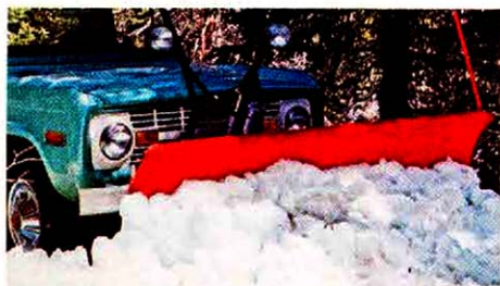
Snowplow Blade may be adjusted easily to various heights and angles (with kit) from within the cab.
