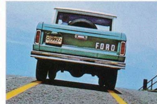
Stability . . . A wide 57.4-in. track for Bronco's front and rear axles reduces side sway on the highway and provides trail-hugging stability when traversing steep hills.
