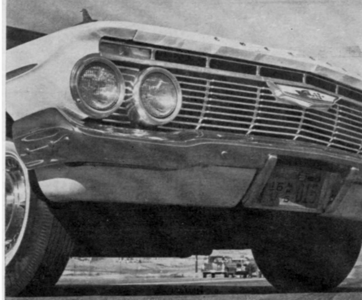
Dual headlights flush with grille line and license plate set in compartment under bumper presents blunt but clean front end.
