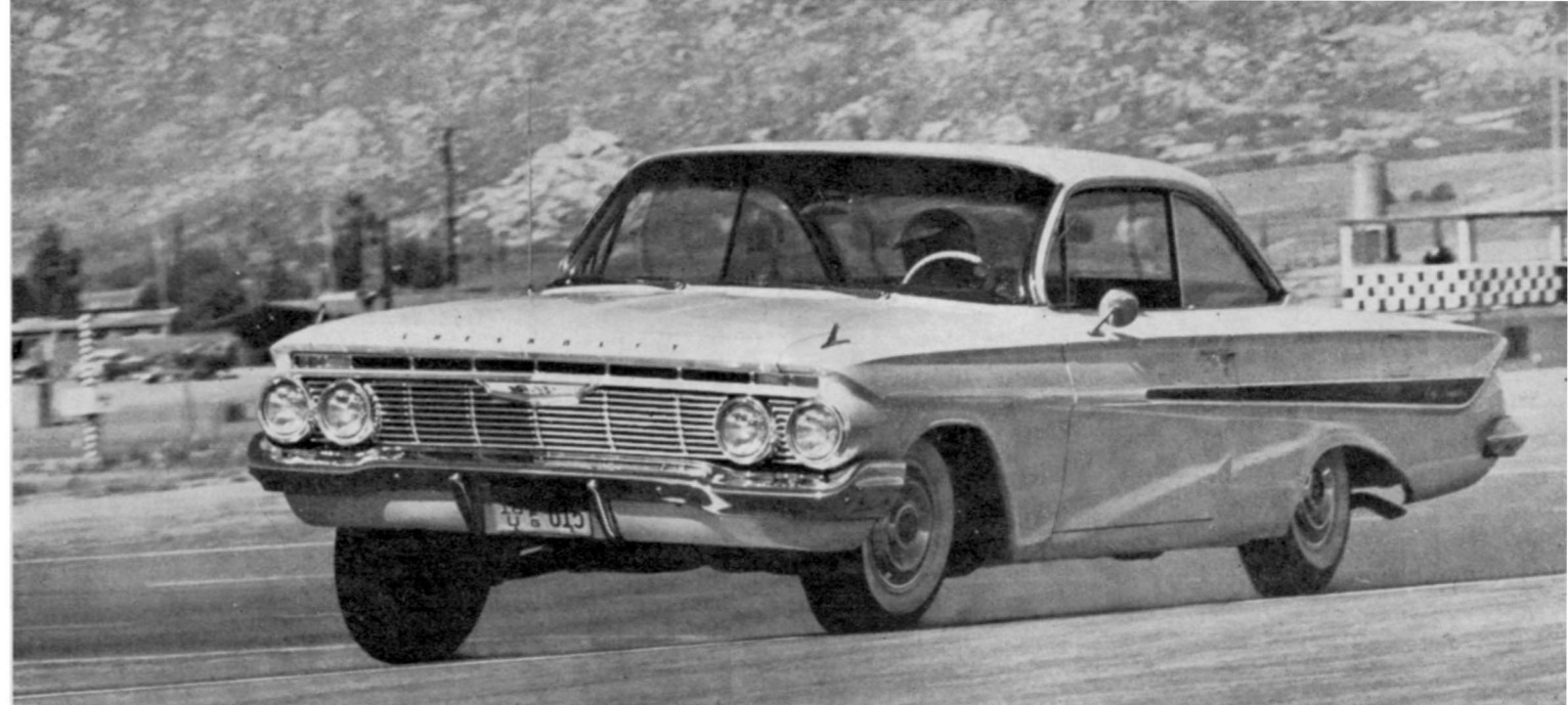
UNDERSTEER AND BODY LEAN ARE ON THE SEVERE SIDE UNDER HARD CORNERING CONDITIONS BUT TIRES STICK WELL, SQUEAL LITTLE.
