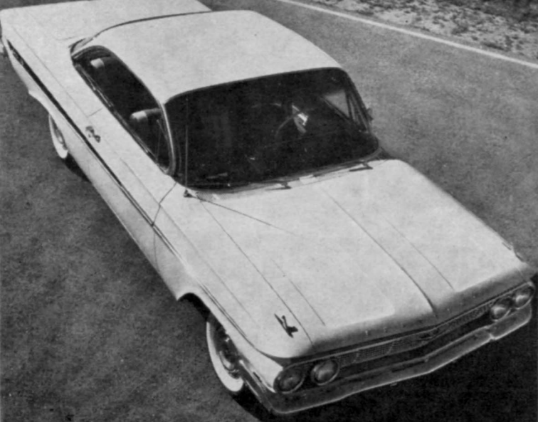
Sculptured pattern stamped in hood panel breaks up wide area of sheet metal without use of chrome trim, increases rigidity.
