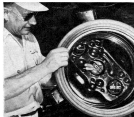
Large diameter air cleaner/silencer with resin-impregnated paper filter cuts drag strip speed seven mph, adds second to ET.
