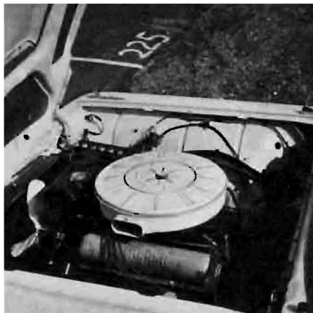
Low, wide engine compartment gives more room to work on 352 and 430 cu. in. mills; both sit far forward.
