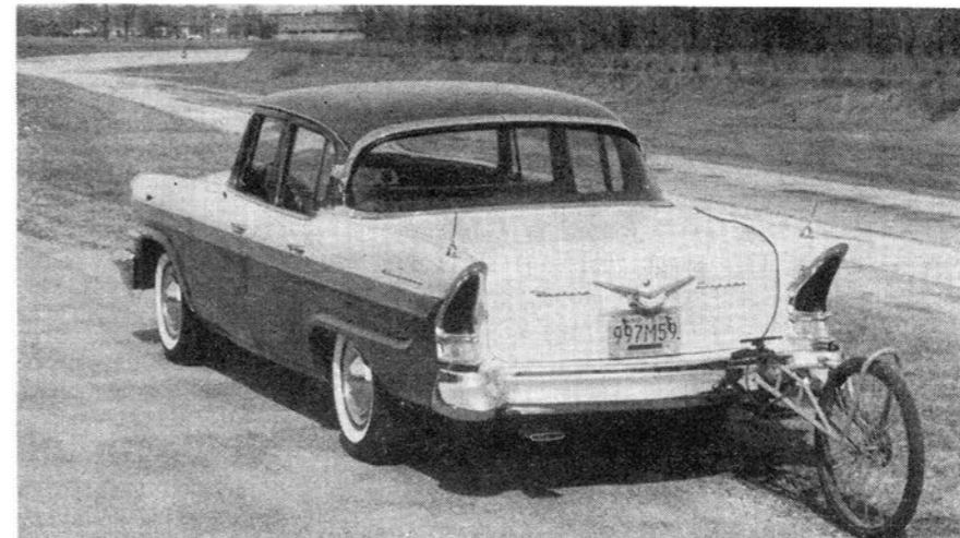
FIFTH WHEEL is used during road tests to assure accurate results. Factory "customizing" job on Studebaker shell makes Packard stand out from lower priced Studebaker sedans.
