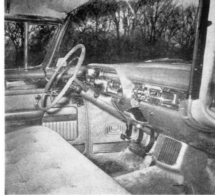
INTERIOR features are very lush and somewhat dazzling to many people. Instruments are grouped in front of the driver and hooded to prevent glare. Radio speaker is mounted below dash in the center.
