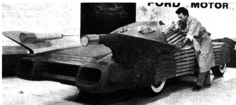
Clay modeler John Ebejer works with rendering as backdrop. Location of oil cooler on lower front fender edge and provision for an after-cooler with grille-work in rear deck lid of car is interesting and may be especially significant.
