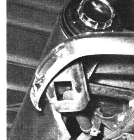
Fewer right angle bends in tail pipe cut back pressure as compared to '55 system. Exhaust is partially deflected by bumper.
