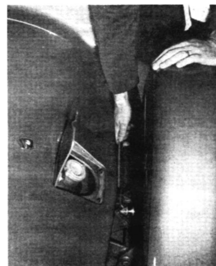
Continental tire mounting must be swung back out of way to permit access to gas filler pipe on the 1956 T-Bird.
