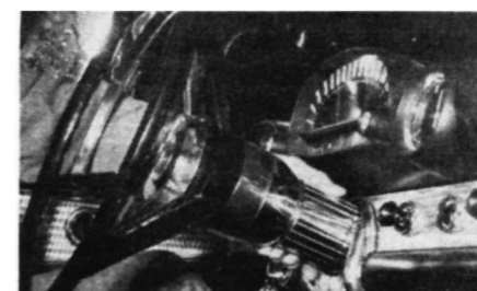
Like predecessors, new T-Bird has an adjustable steering wheel. Turning of a knurled collar locks wheel in position.
