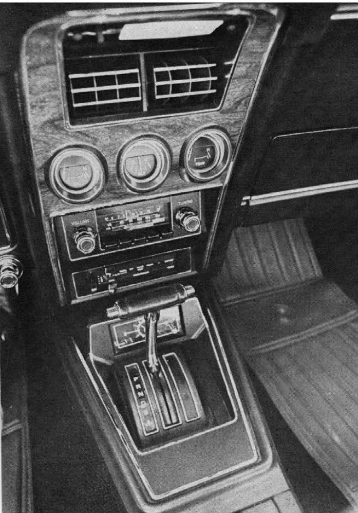
Above: The center console of the Mach I and Boss 351 models contains a full range of gauges, a detail which the hardtop lacks. Only the electric clock, partially covered by shift lever, is hard to read without removing gaze from the road.
