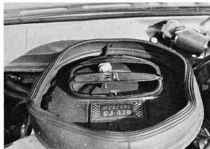
Vacuum-controlled flap lets in cool fresh air for max perf when throttle is floored.
