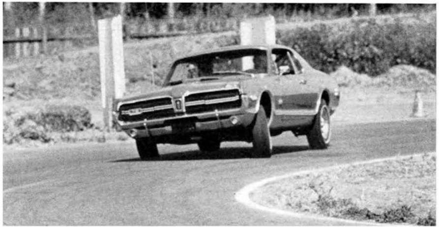
OPTIONAL SUSPENSION did not reduce incredible understeer of Cougar XR-7. Angle of front wheels relative to vehicle direction graphically demonstrates lack of steering effectiveness. Wheels turn, but Cougar refuses to answer the helm.
