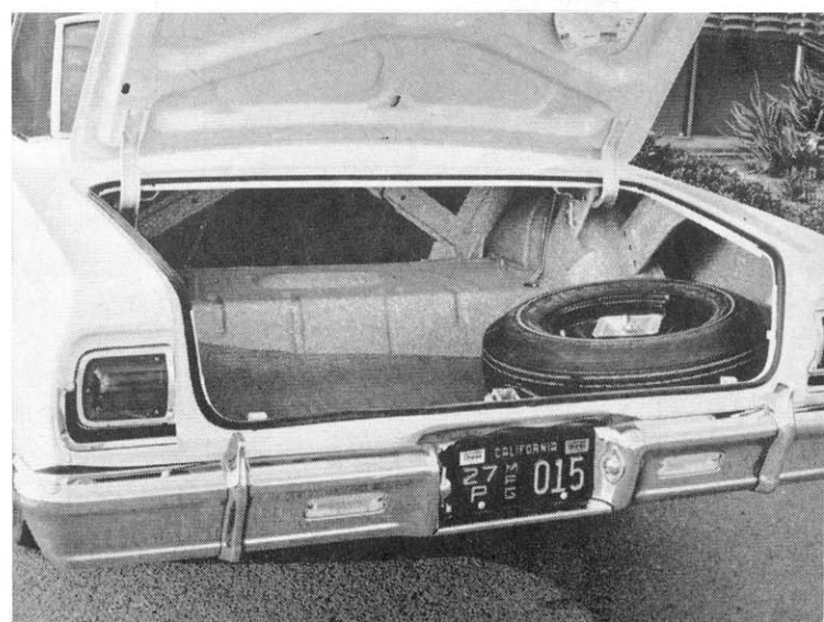
GENEROUS-SIZED trunk of Chevelle could be equipped with a concrete floor mat to counterbalance over-heavy front end.
