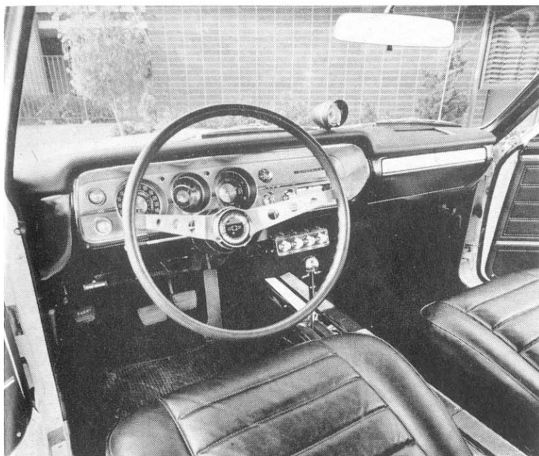
INSTRUMENT PANEL features full set of gauges, tachometer in middle. Stereo controls are just above shift-lever.
