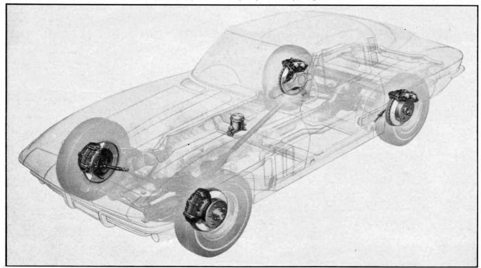
the driver could provide sufficient line pressure for all the conditions of lining frictional properties, a vacuum booster was considered necessary. The result of all this was, as we said, a superb brake system—derived from drums and various crutches, and necessarily very expensive.
