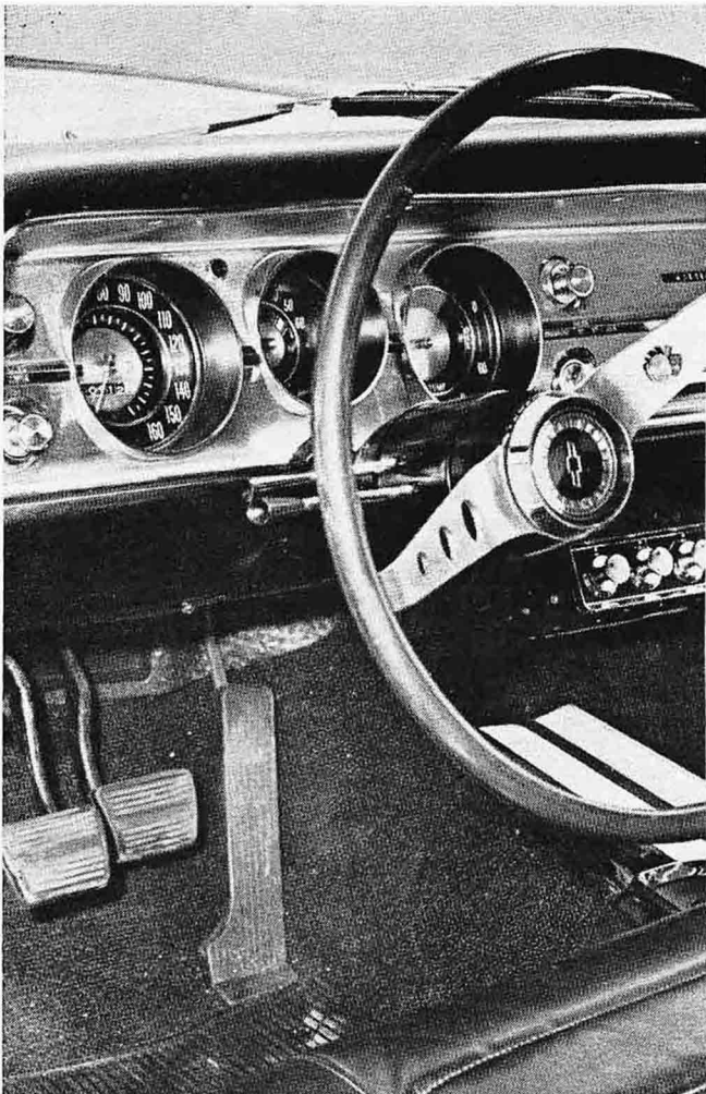
160-mph speedometer, on left, isn't there just for window dressing (see text). Easy-to-see tach occupies the center slot.
