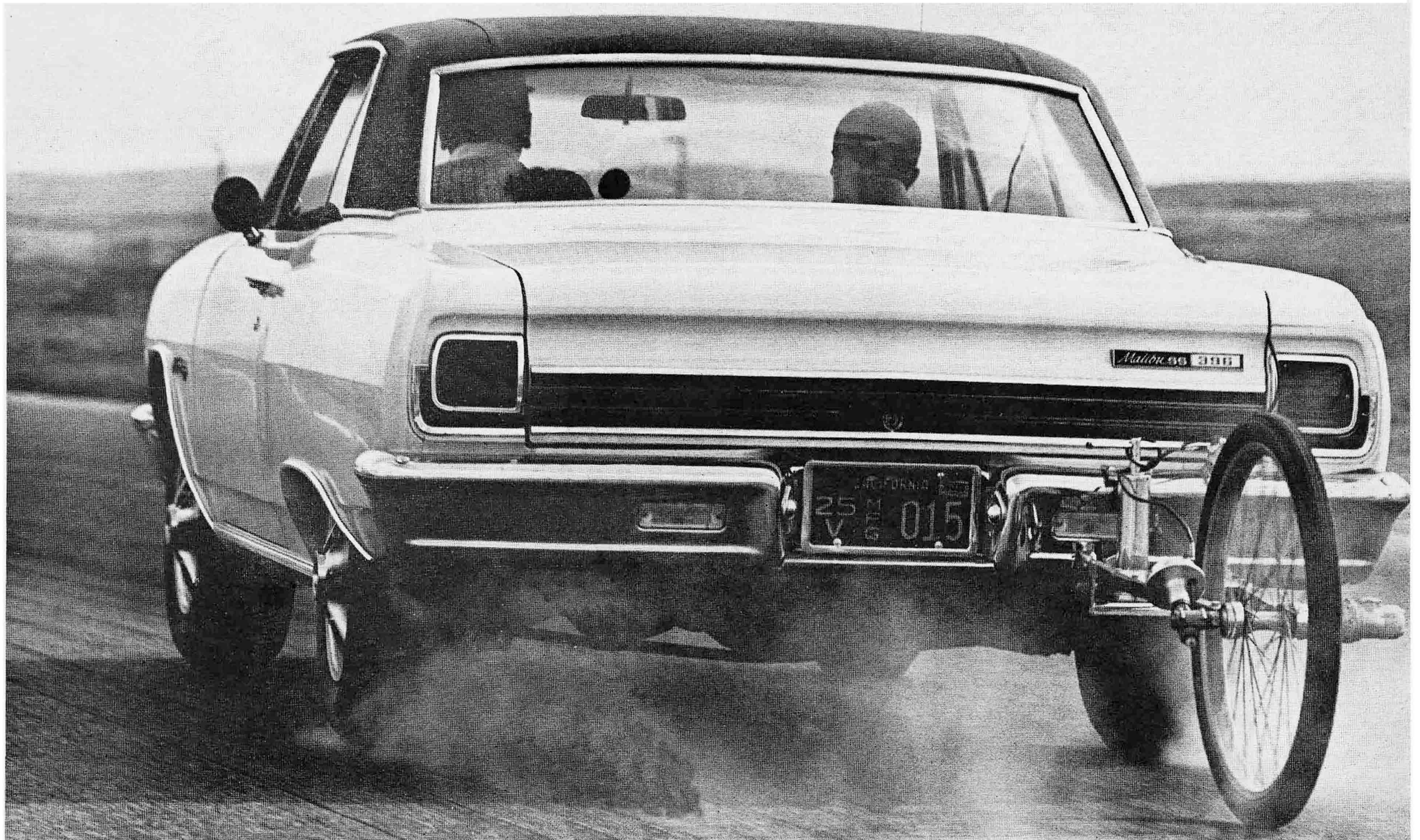
(RIGHT) Charging off line with both rear tires smoking got lowest times. New suspension makes this possible without limited-slip differential or locked rear end.
