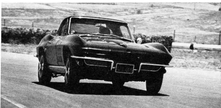
Sting Ray lifts its nose under power and charges out of turns with excellent stability and control. Street tires limit traction.
