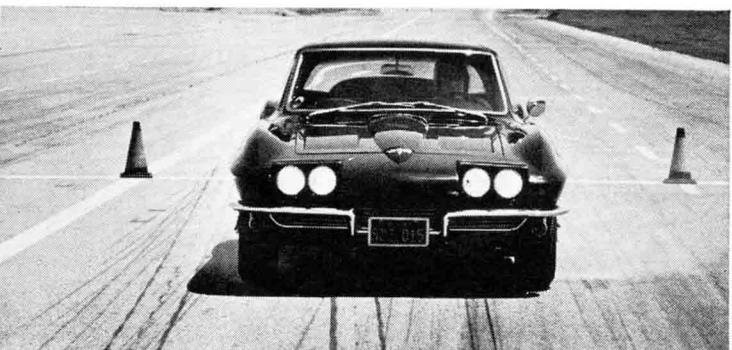
Quick stops were Corvette's forte when equipped with special brake option. Some nose dive was evident, but car kept all four wheels on the ground, held down swerve and fade to a minimum.
