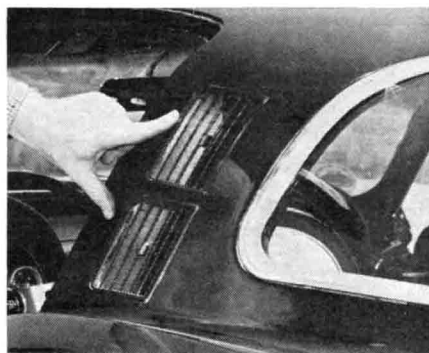
Ventilation blower exhausts stale inside air through left vents for greater comfort.
