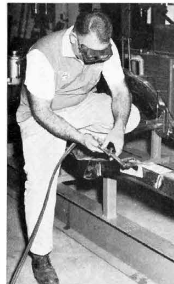
SPECIAL JIGS guide Stroppe's torch, hold frame in alignment during construction. Above right: Louis Unser turns differential housing in lathe after welding on safety hubs. Below: Extra straps criss-cross fuel tank to provide additional support.
