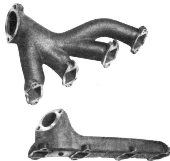
OVERALL VIEW of Ford's 352-cubic-inch V-8 equipped with the Interceptor option is almost too tame to give the impression that this is the home of 360 horsepower. Note how the cast-iron manifolds (top) resemble tubing headers in their shape. Latter were used in development of this engine.
