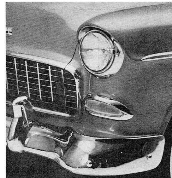
Frontal treatment of the 1955 Chevrolet features inward slope, Ferrari-type grille, hooded headlights and wrap-around bumper.
