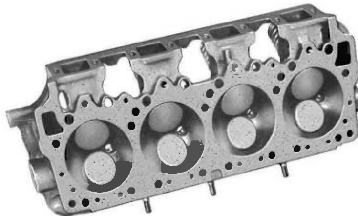
HEMISPHERICAL COMBUSTION CHAMBERS — 1964 CHRYSLER CORPORATION MAXIMUM-PERFORMANCE ENGINES
