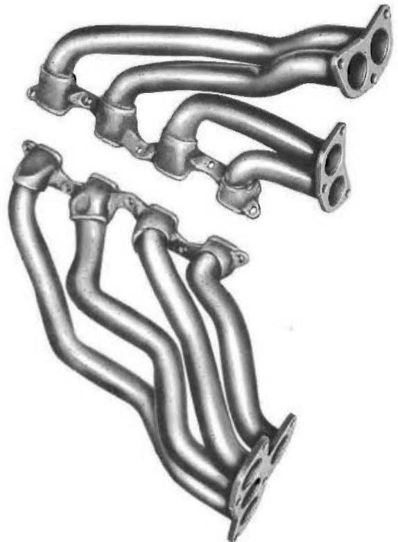
EXHAUST HEADERS — 1964 CHRYSLER CORPORATION HEMISPHERICAL - CHAMBER, MAXIMUM - PERFORMANCE ENGINES
