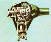
POSITRACTION REAR AXLE! This extra-cost option enables the El Camino to handle on or off-the-road hauls with ease. Positraction directs the power to whichever wheel is getting the best traction. It helps wheels to grip on any road surface for safer control.
