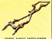
STURDY X-BUILT SAFETY-GIRDER FRAME. All-welded box section side members and box girder center beam give rigidity that resists strains from maximum loads and rutty roads. Tough frame is a solid reason for high 4,900-lb. maximum G.V.W. rating.
