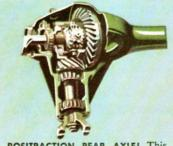
POSITRACTION REAR AXLE! This Camino to handle on or off-theroad hauls with ease. Positraction directs the power to whichever wheel is getting the best traction. It helps wheels to grip on any road surface for safer control.
