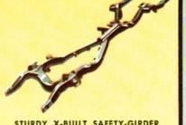
STURDY X-BUILT SAFETY-GIRDER FRAME. All-welded box section side members and box girder center beam give rigidity that resists strains from maximum loads and rutty roads. Tough frame is a solid reason for high 4,900-lb. maximum G.V.W. rating.
