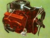
MODERN SHORT-STROKE V8 POWER. Two up-to-the-minute V8's complement the advanced styling of the El Camino. Fast-stepping, economical performance is provided by either the smooth 185-h.p., 283-cubic-inch Turbo-Fire V8 . . or the mighty 230-h.p. Super Turbo-Fire V8\*.
