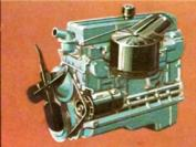
for fuel, lower driving costs, stem from new Hi-Thrift 6 advance-ments. New camshaft design, for instance, can improve gas econ-omy by as much as 10% and it gives the engine greater torque (more pulling power). Hi-Thrift 6 is rated at 135 horsepower.
