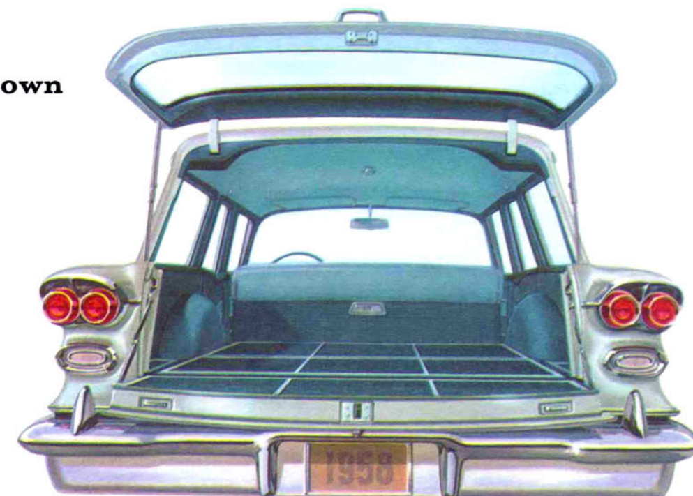
Deep goes the cargo space in a Safari—over 9½ feet, with tailgate down! New wrap-around lift-gate gives you greater loading ease, swings high out of the way to afford a full 30-inch-high opening, locks "open" in six different positions. Star Chief Safari optional interior and carpeting shown.
