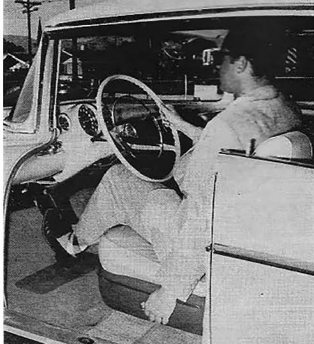
Access to the driver's seat is good, but the seat doesn't adjust far enough to the rear. Tall people will bump their knees on the steering wheel.
