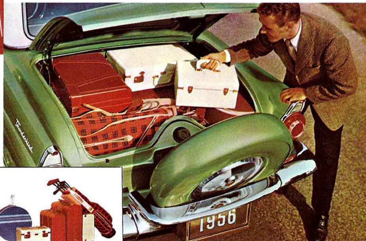
With the spare tire mounted outside , there's space for all the luggage you see at left, and more, in the Thunderbird's big new luggage compartment. New spare tire mount moves back out of way on hinged bracket. Deck-lid pops open on counterbalancing hinges when you turn the key.
