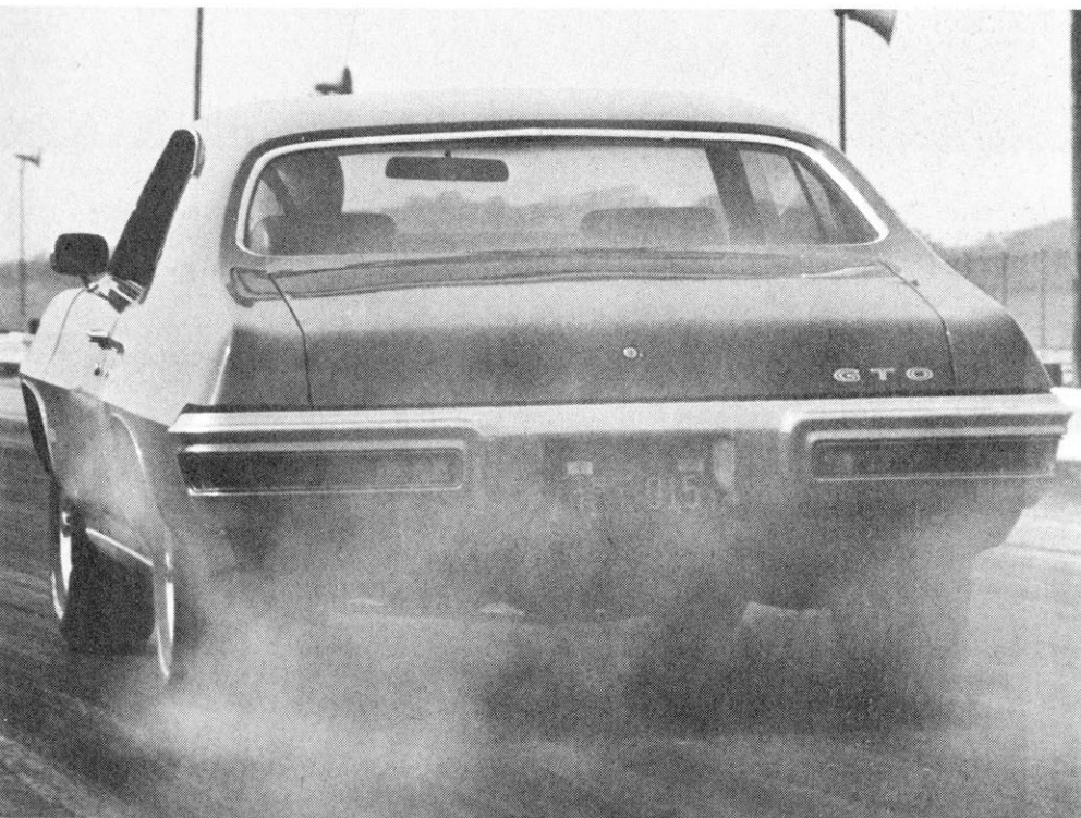
Our best drag time was a 14.50 ET at 97.76 mph, but POP ROD feels that with the proper gear and tuning the "Goat" could easily run in the 13-second bracket. Trying not to break the Uni Royal G70 X 14 tires loose seemed to be the problem of the day.
