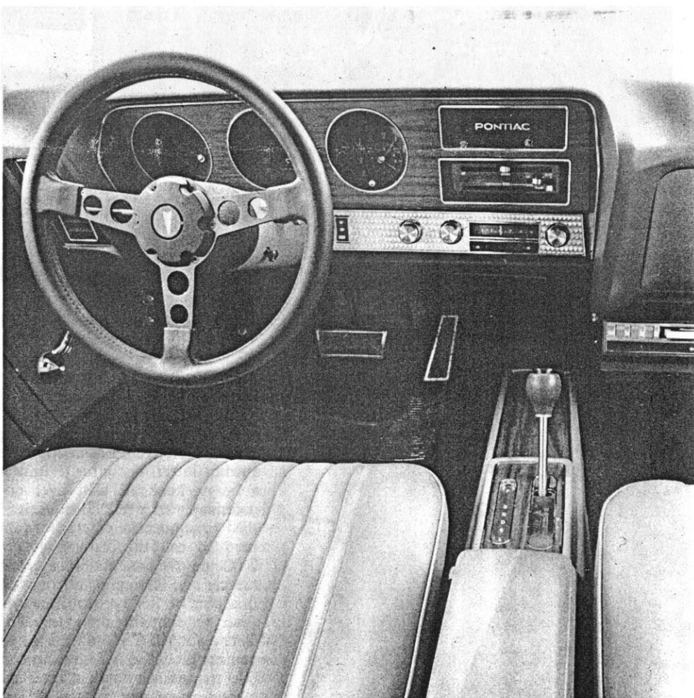
Uncluttered dash is decorated with nice thick rimmed steering wheel (optional) and Ampex tape deck (also optional).
