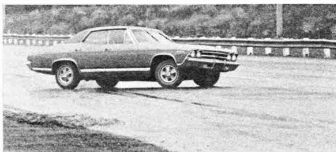
SCARY MOMENT came when Chevelle locked one wheel during brake test, and spun the car half-way around. The flaw was the fault of the one car, but Chevrolet's high-boost power brakes magnified it. The light pedal is difficult to modulate.
